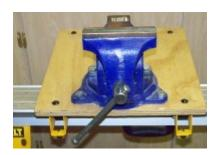
**Table for the sturdy and heavy British Vice**. The British vices are my favorite. Simple, rugged and the cast iron is perfectly made. On the rear of this table a bench-top grinder (Ryobi) can be attached. As the vice is already extremely heavy it isn't a good idea to have it permanently there.
